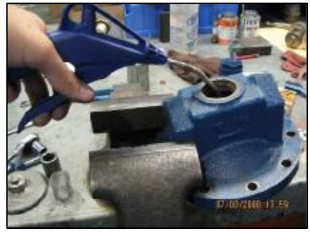
Blow debris from body & reassemble.
