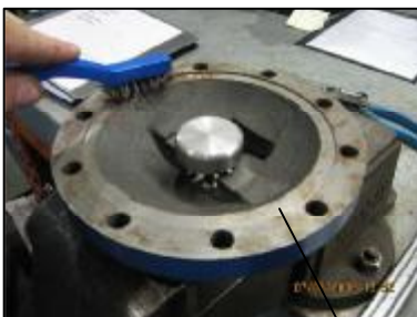
Clean gasket surfaces.
